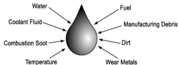
*There is a need for a consistent, high-quality, real-time, cost-effective oil condition sensor that measures and reports chemical degradation, total contamination and water content in oil, as well as oil temperature, all simultaneously in a single unit.*
